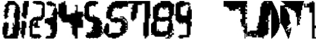
Figure 3. Some blobs. The first ten show blobs that belong to digits. The right section shows non-digit blobs found after filtering. Note that we find both polarities (white on black and black on white) of digits, we convert them to black on white for display purposes. Also, note that corners and edges can pop up similar to the digits 7 and 1.
