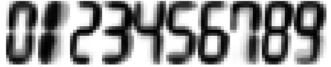
Figure 4. "Average" digits, reflecting the probability of a pixel being on/off for a given digit.
