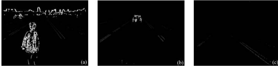
Fig. 10. Examples of disparity map of the vehicle environment (a) under sunny weather, (b) under foggy weather, and (c) under dense foggy weather before nightfall. White points are considered as obstacle points. The gray level of other points is proportional to their disparity.
