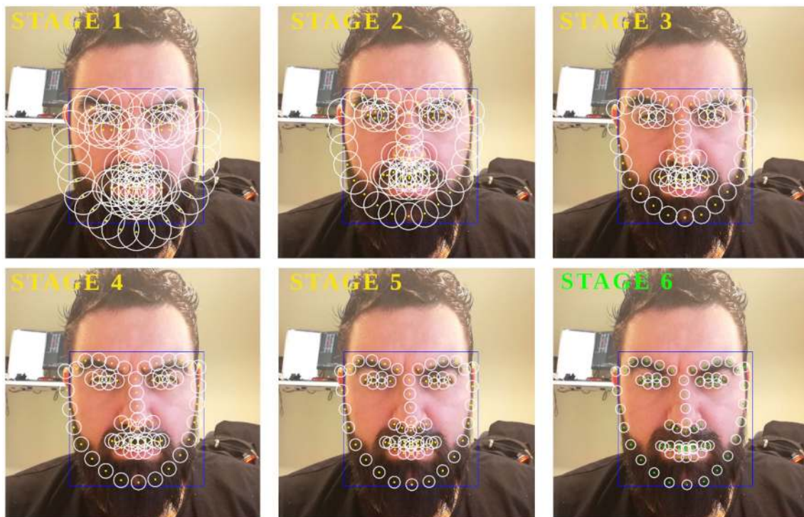
Fig. 3 Stage-by-stage process in the LBF method. The searching area (local region) around each landmark and the radius for each stage decreases along the cascade [18]
