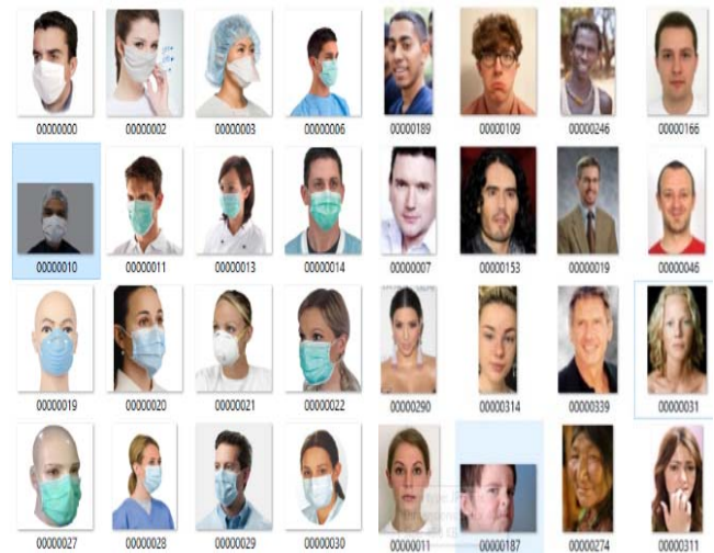
Fig. 3. Annotated Image data collection of the proposed computer vision to detect facemask with a person wearing and not wearing a facemask
