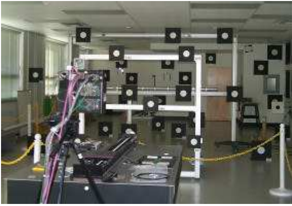
Figure 6. Experimental setup used to verify the accuracy of the tracking system. The blinds were shut to prevent saturation in this photograph.
