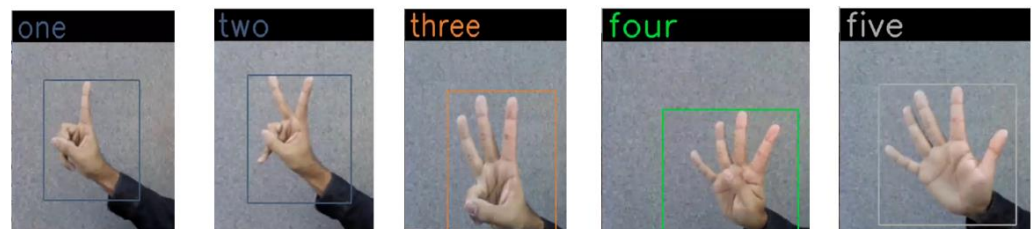
Figure 7. Gesture detected using the proposed YOLOv3-based methodology.
