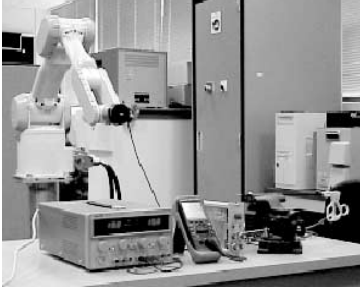
Fig. 4. Calibration setup for the strain gages on the force sensing forceps.
