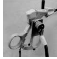
Fig. 3. Position sensor attached to the laparoscopic tool.
