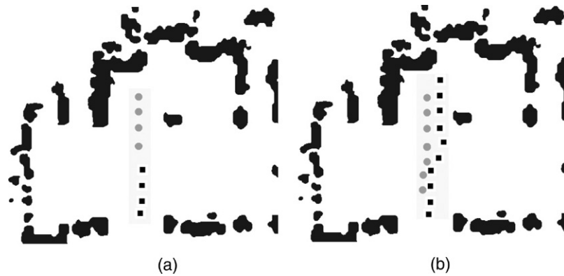
Fig. 7. Two snapshots (a)–(b) of a navigation session for avoiding a human to reach the goal position. The robot track is marked with the black squares (■) and the human track is marked with the grey dots (●).
