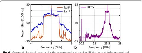
**Fig. 6** Measured electrical spectra of **a** the transmitted and received IF signals and **b** the transmitted mm-wave RF signal. IF: intermediate frequency, RF: radio frequency
