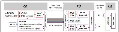
**Fig. 3** Fronthaul architecture with CO, ARoF fronthaul over SDM based ODN, RU and mm-wave 5G NR air interface to the end user. CO: central office, RU: remote unit, UE: user equipment, ARoF: analog radio-over-fiber, SDM: space division multiplexing, ODN: optical distribution network, 5G NR: 5G new radio, RF: radio frequency, IF: intermediate frequency, BBU: baseband unit, DSP: digital signal processing, LO: local oscillator, MCF: multi-core fiber, DL: downlink, UL: uplink
