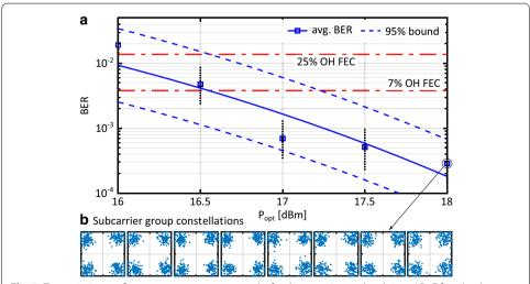
**Fig. 7** Transmission perfromance measurement results for the experimental real-time ARoF fronthaul demonstration: **a** real-time BER in dependence of optical power after two-tone generation and associated statistics, **b** observed constellations for the 800 MHz wide 5G NR OFDM signal. BER: bit error rate, OH: overhead, FEC: forward error correction
