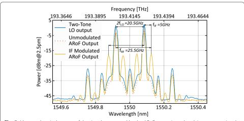
**Fig. 5** Measured optical spectra of the signals generated by the ARoF transmitter: the plain two-tone signal output used for the remote-fed LO, the ARoF signal before and after modulation with the IF signal
