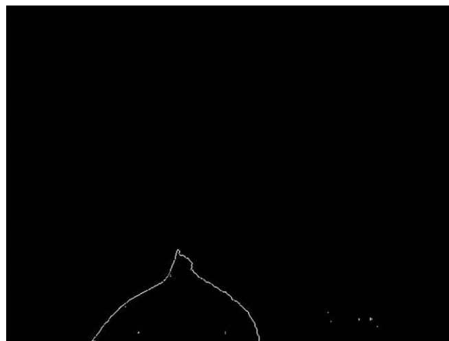
Fig. S5. Traced notch/crack profile by applying the Sobel method.
