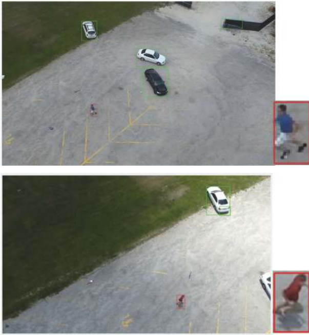
FIGURE 10: Humans running in the UCF-ARG dataset: the green boundary boxes in the image are the results after using optical flow. The red boundary boxes are the results after applying human classification based on deep models.
