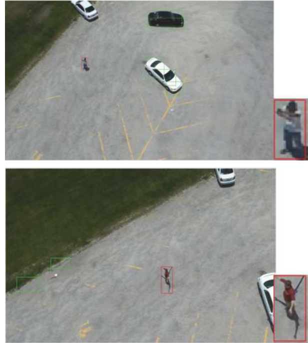
FIGURE 11: Humans waving in the UCF-ARG dataset: the green boundary boxes in each image are the results after using optical flow. The red boundary boxes are the results after applying human classification based on deep models.
