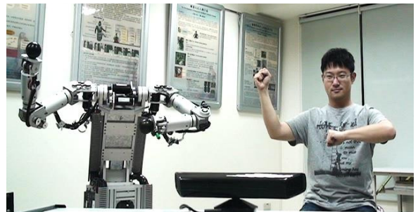
Fig. 1. The robot is controlled by human demonstration in real time using Kinect sensor.
