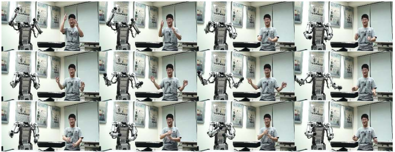
Fig. 13. A sequence of photos shows the robot imitates human motion in real time. (Take three shots per second.)
