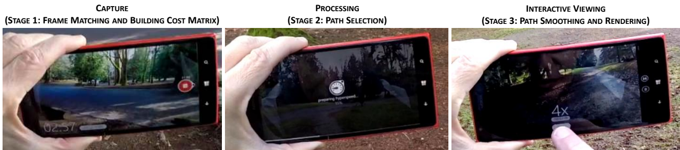
Figure 4: Our smartphone app and the three stages of our algorithm mapped to the user experience. Stage 1 occurs online during capture, Stage 2 is a short processing stage following capture, and Stage 3 occurs online during interactive viewing, where a user can use an on-screen slider to immediately change the speed-up for the displayed hyperlapse.
