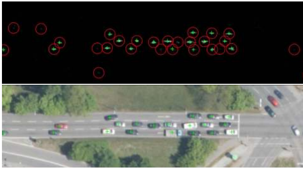
Figure 3: Upper: Confidence image with detected blobs (red circles) and final SVM detection (green crosses). Lower: Original image with final detection.
