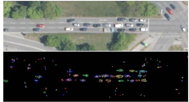
Figure 2: Upper: Horizontal aligned original image. Lower: Confidence image with zero crossing.
