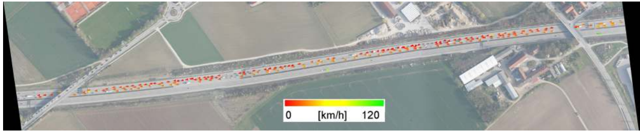
Figure 6: Traffic data extracted automatically by the processing chain on BAUMA campaign 2010 near exit "Munich exhibition center" of motorway A 94. Quality of traffic data is 80 % in case of that campaign. Periodic gaps in traffic data are due to missing overlap between image bursts (which can be corrected easily by flight planning in future campaigns).
