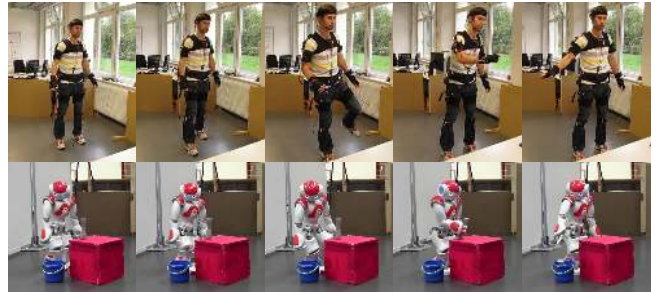
Fig. 11. Tele-operated walking and object manipulation. The complete motion sequence is contained in the video accompanying this paper.
