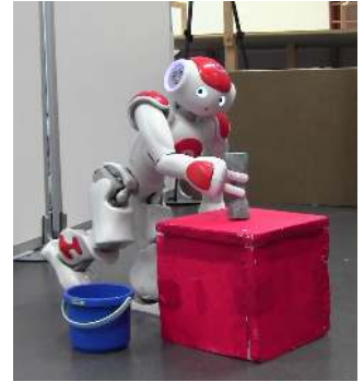
Fig. 1. Imitation of a complex whole-body motion with a humanoid for a tele-operated manipulation task. Note that the robot imitates configurations in which it is required to balance on one foot over a longer period of time.
