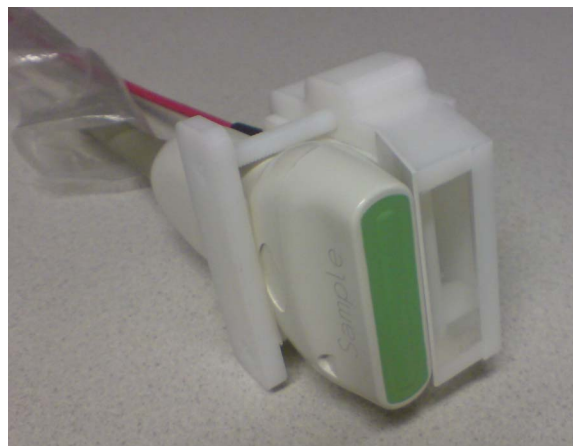
Fig. 1 Optical system attached to an existing ultrasound probe.
