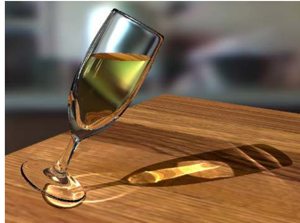
Figure 1: GPU ray tracing and photon mapping for a dynamic scene, where both the scene geometry and the light source can be changed. Two kd-trees are built from scratch for each frame, one for the scene geometry and the other for the photons. Shadows, reflection/refraction, as well as caustics caused by the glass and champagne are rendered at around 8 fps for 800 \times 600 images.
