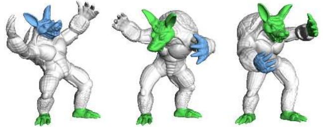
Figure 9: Deforming a point cloud (170K points). The active handle is marked in blue. Our algorithm allows the user to define and switch to new handles quickly.
