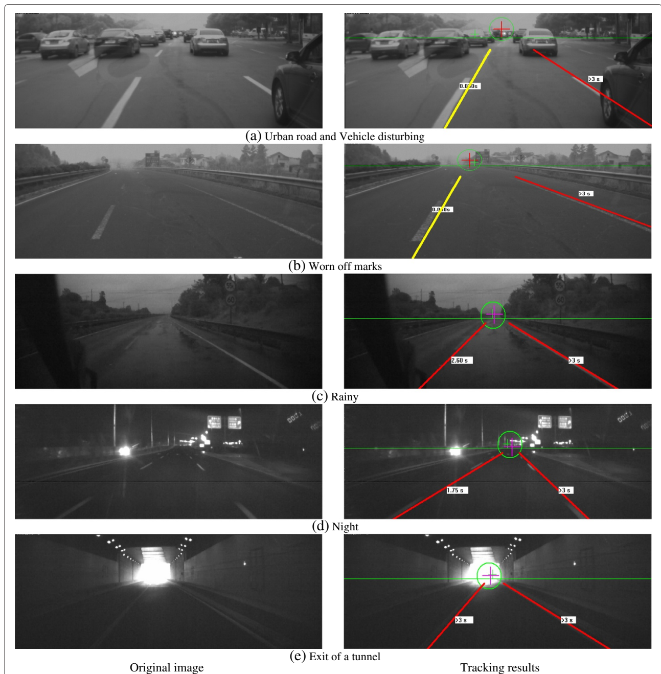
Figure 13 Actual road experiments. Results in various scenarios. (a) Urban road and vehicle disturbing. (b) Worn off marks. (c) Rainy. (d) Night. (e) Exit of a tunnel. In the left parts are the original images. The small cross in the right parts denotes the position of the vanishing point, and the circle around the vanishing point represents the parameter space range of \rho = 4\sigma . Red line means the tracked lane marking, and warning time is tagged beside the marked lane. Yellow line means the alarm is triggered.
