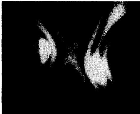
Figure 4. Fringe pattern of an oscillating loudspeaker at 500 Hz.
