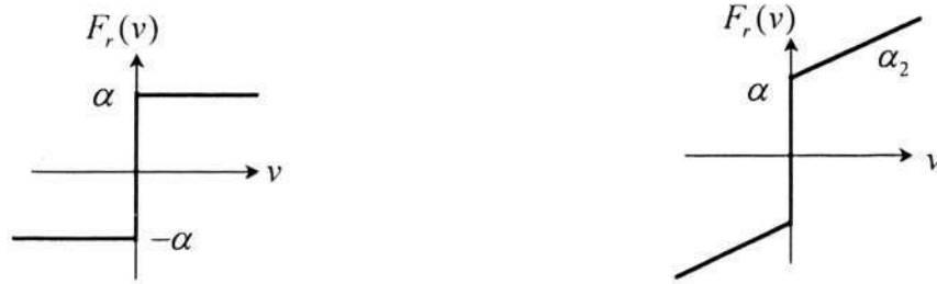
Fig. 2-4 Plot of (a) Coulomb friction and (b) Coulomb + Viscous friction versus velocity;
