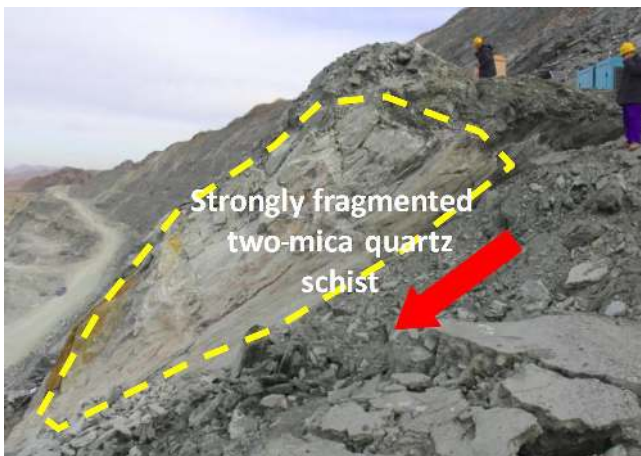
Figure 4. Slip surface consisting of strongly fragmented two-mica quartz schist.
