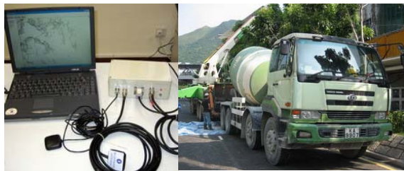
Fig. 3 Prototype of the RMC monitoring system and site trials on the truckmixer
