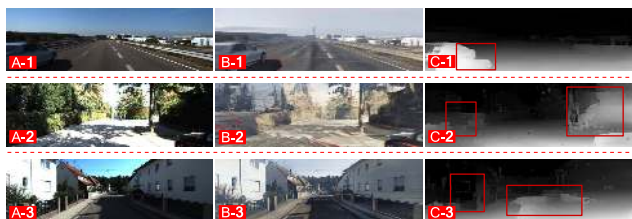
Figure 9: Examples of failures, mainly due to light saturation and shadows. Issues are marked with red boxes.
