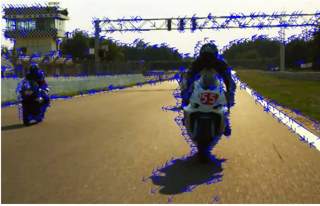
Fig. 4. An example part of the Full HD video frame with characteristic points detected with the Harris corner detector and then tracked with the Lucas-Kanade method. Displacements are marked with arrows. Note that the arrows located on the static objects like trees or a building are there as a result of moving camera
