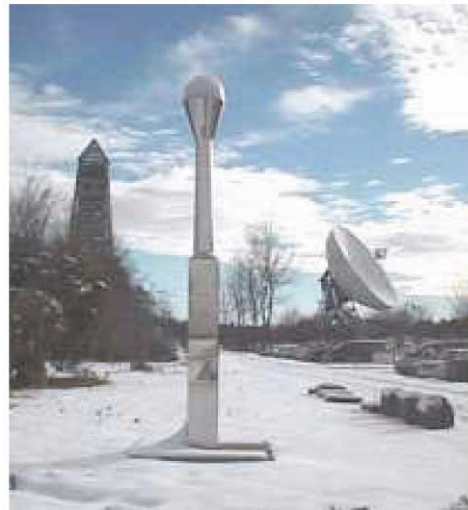
Fig. 11. GPS network sites in Japan are housed in 5 m tall stainless-steel towers, as shown. The sites are maintained by private companies under contract; communications are provided by telephone.
