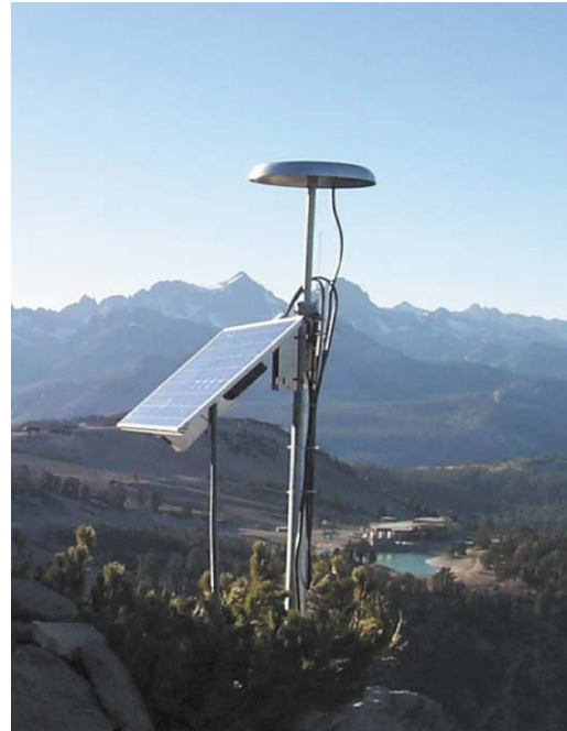
Fig. 9. An L1 receiver system deployed for volcano studies at Long Valley, CA. The system, including solar power and a radio modem communication link, was developed by the UNAVCO Facility ( www.unavco.ucar.edu/science_tech/volcano/11 ). Hardware cost for this system is less than $4000.
