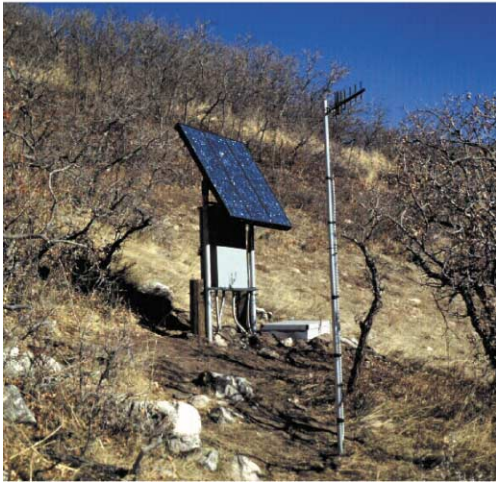
Fig. 13. A solar-powered GPS site with radio modem telemetry established by the University of Utah for atmospheric and geodetic applications, with assistance from UNAVCO. The site is located in a geologically stable location with a radio telemetry link to campus. The enclosure beneath the solar panel contains GPS receiver equipment and batteries. Similar installations are expected for universities interested in combined atmospheric and geodetic applications.
