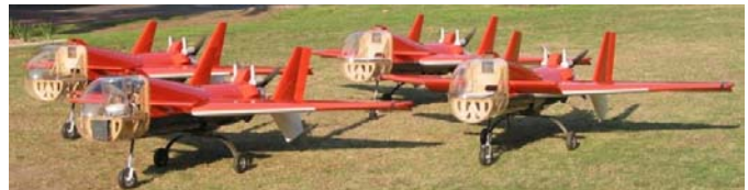
Fig. 3. The four flight vehicles: MK3-Brumby. Four sets of identical GNC modules are installed on the vehicles with different mission load.
