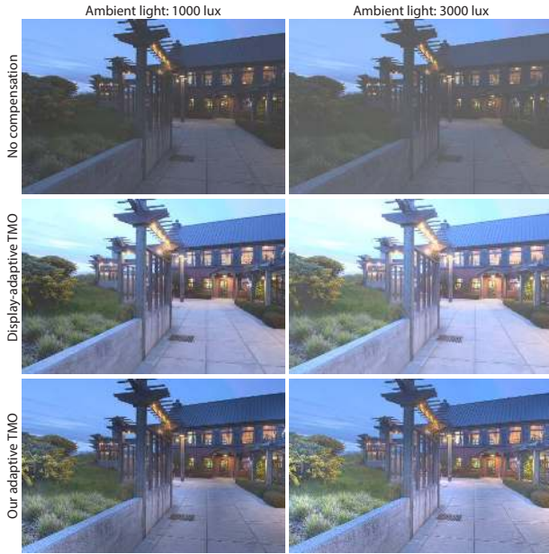
Figure 15: The effect of ambient light on the results of tone-mapping. Top-row: our method disregarding ambient light; middle row: display-adaptive TMO [Mantiuk et al. 2008]; bottom row: our method adapting to ambient light. The image contrast (dynamic range) is the same in each column. Simulated display: black level: 1 cd/m 2 ; reflectivity: 1%; peak lum.: 100 cd/m 2 . Notice the difference in detail visibility.
