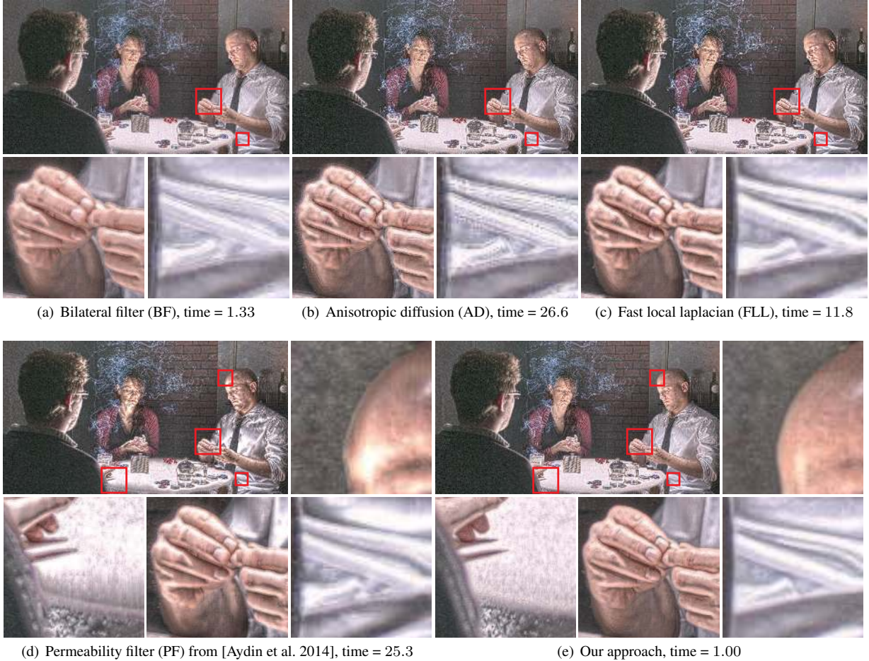
Figure 9: The figures use the same tone curve, but different edge-preserving filters for detail extraction. The details are scaled by a factor 5 to highlight filtering differences and artifacts, and enlarged versions show the areas indicated by the red squares in the images. Timings of Matlab implementations of the filters are also given, compared relative to our approach.
