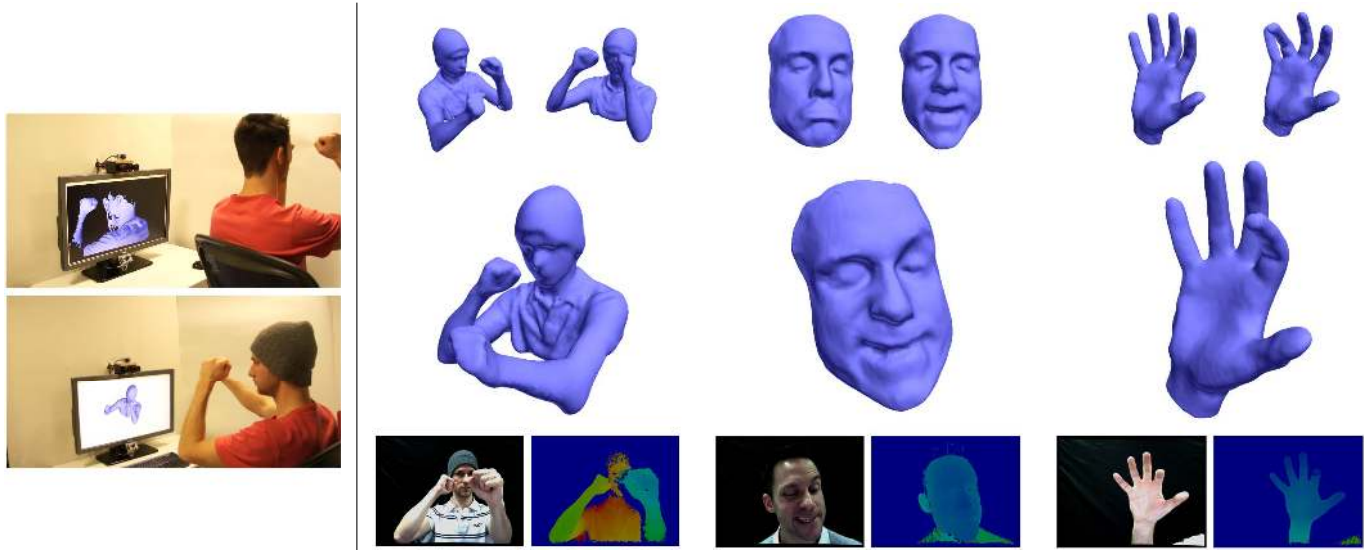
Figure 1: Our system enables the real-time capture of general shapes undergoing non-rigid deformations using a single depth camera. Top left: the object to be captured is scanned while undergoing rigid deformations, creating a base template. Bottom left: the object is manipulated and our method deforms the template to track the object. Top and middle row: we show our reconstruction for upper body, face, and hand sequences being captured in different poses as they are deformed. Bottom row: we show corresponding color and depth data for the reconstructed mesh in the middle row.
