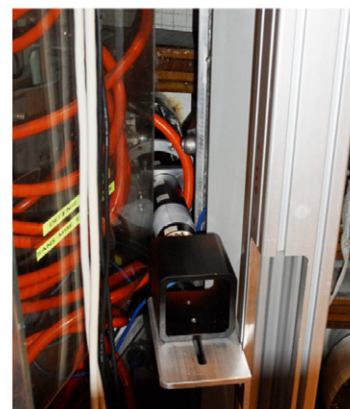
Figure 4. (Left) CAD drawing of tangential port plug, optic and support structure. (Right) Optic installed on the TCV mid-plane tangential port. Also showing magnetic shielding required for reliable operation of the cameras during discharges.
