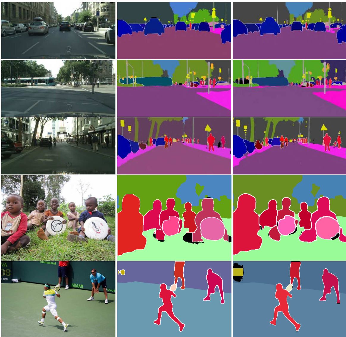
Figure 4: Panoptic segmentation results on CityScapes and COCO comparing our predictions and UPSNet [36]. We leave it to the reader to guess which results are ours (the answer is in [1]).
