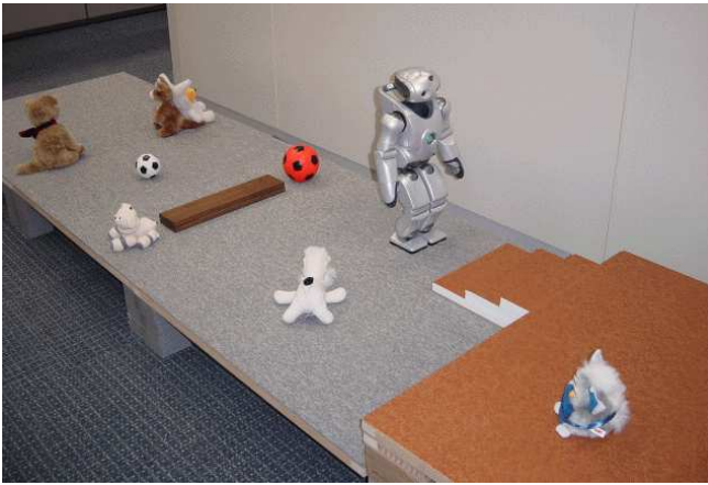
Figure 5: Experimental setup. Several obstacles and a sill are placed on a stage. A staircase leads to a higher-level platform.
