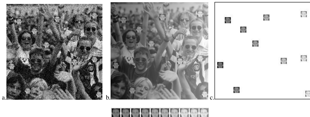
Figure 10: An original image was embedded with 10 occurrences of a pattern. a) Noise was added to the image at a level of 40 (see text). b. A gradient of illumination was added to the image. The 10 patterns as appearing in the image are shown below. c. All 10 patterns of varying illuminations were found. Five projections were required to find all 10 patterns.
