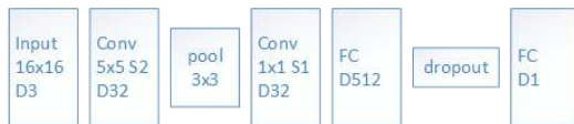
Figure 3: The architecture of the tiny deep network for pedestrian detection, which is a part of the DNN cascade.
