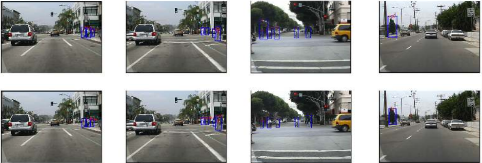
Figure 6: Example detections of the Fast Cascade of DNNs on the Caltech test data. The top row corresponds to detections with a model trained on Caltech data, the bottom row is for a model trained on Independent data. Interestingly, the two models often make similar mistakes, although they are trained on non-overlapping datasets (see the right-most column).
