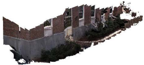
Figure 7. The reconstruction produced by our algorithm from several hundred frames of video. By testing only plane hypotheses with high prior probability, the reconstruction was achieved with only 48 plane hypotheses per frame at a speed of 20.0 Hz.
