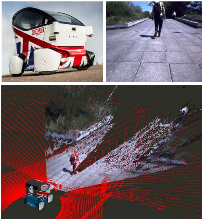
Fig. 1. Real-time fusion of stereo and LIDAR range data for a small autonomous vehicle “Pod” operating in urban environments. The vehicle (top left) is equipped with multiple low-cost 3D LIDAR scanners and a stereo camera. Images from the camera (top right) are fused in real-time with sparse 3D LIDAR points (bottom, red) to form a dense depth map (bottom, coloured) suitable for online localisation, mapping, path planning and obstacle avoidance.
