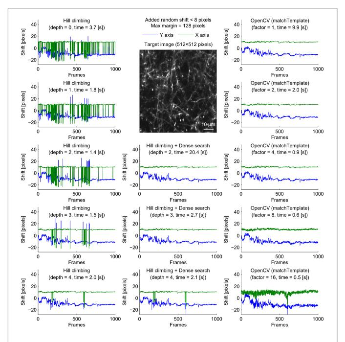
FIGURE 4 | Comparison of speed and stability with different algorithms and parameters with artificially added random shifts for dendrite imaging. Same as Figure 1 applied to dendrite imaging with random shifts (up to 8 pixels in each direction) added artificially before motion correction. For visualization, these artificially added shifts were subtracted before the corrected distances are plotted.
