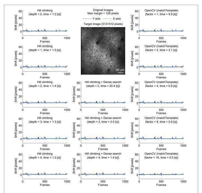
**FIGURE 1** Comparison of speed and stability with different algorithms and parameters for neural ensemble imaging. Estimated shifts (blue: Y axis, green: X axis) with different algorithms and parameters for cell body imaging (512 × 512 pixels, 1000 frames). Dense search was slowest even at depth = 2 and shallower depth was not included.). Maximum shift for correction was set to be 128 pixels in all conditions.
