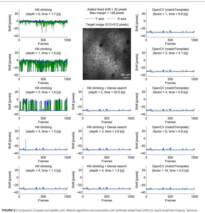
Figure 1 with fixed shifts (32 pixels in both X and Y axis) added artificially before motion correction.
