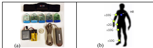
Figure 1. (a) Five 3-axis wireless accelerometers, a heart rate monitor, and USB wireless receiver, and (b) Placement of the sensors on the body.
