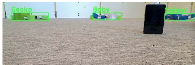
Fig. 4: The recognition of three modular robots. The left is ‘Gecko’. The middle is ‘Baby’. The right is ‘Spider’. The green texts above bounding box are the names of recognized robots. The green bounding boxes are the regions of recognized robots. The black box occludes a piece of ‘Spider’. please note that black color is not a color feature of the modular robots ‘baby’.
