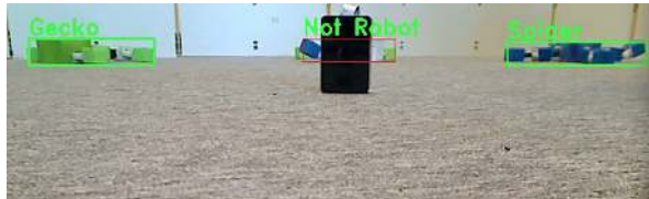
Fig. 5: The recognition for an occlusion situation. The center part of robot ‘Baby’ (middle) is occluded by a black box. The red bounding box is the ROI proposed by FROIS algorithm. The green text above the red bounding box is ‘Not Robot’.
