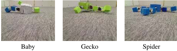
Fig. 2: Images of three real moving modular robots with different morphologies. The ‘Baby’ has 8 components in blue, white, and green color. The ‘Gecko’ has 7 green components. The ‘spider’ has 9 blue components.
