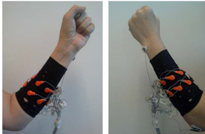
Fig 1. Forearm of a normally limbed subject wearing the textile hose including 16 electrodes.
