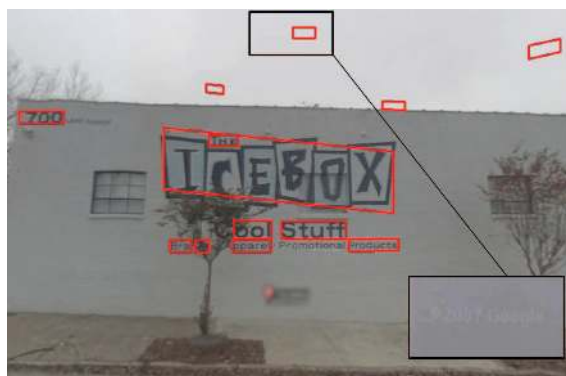
Figure 1. Text detection in the SVT dataset. All “false positives” in the image are caused by watermarks embedded into the dataset. This demonstrates robustness of the proposed method against noise and low contrast of characters (in the bottom-right corner the area of interest is enlarged and contrast artificially increased, “©2007 Google” is readable).
