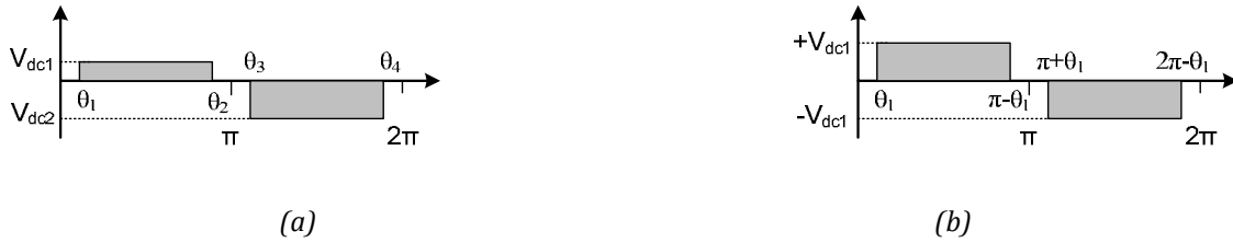
Figure 6 – Generic waveform (a) and H-bridge inverter waveform with quarter wave symmetry (b).
