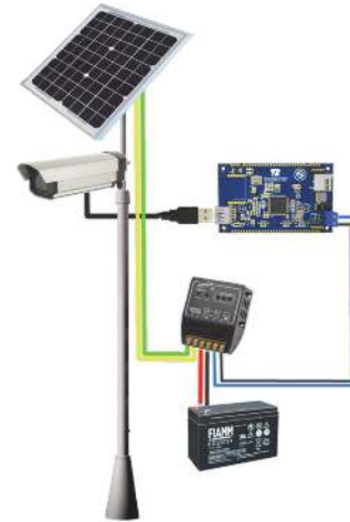
FIGURE 8: VSN sensor node prototype with energy harvesting system.
