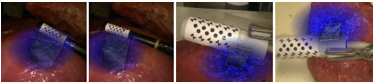
Fig. 9 Ultrasound image is fused with laparoscopic image using an inverse realism technique [19]
