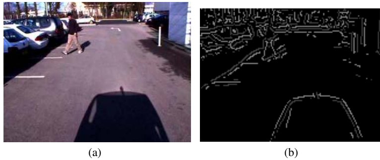
Fig. 3. Gaussian image 3(a) and detected ridges 3(b) at the scale level \sigma = 4 . As we can see, the elongated shape, as the legs or the ground lines are well detected.
