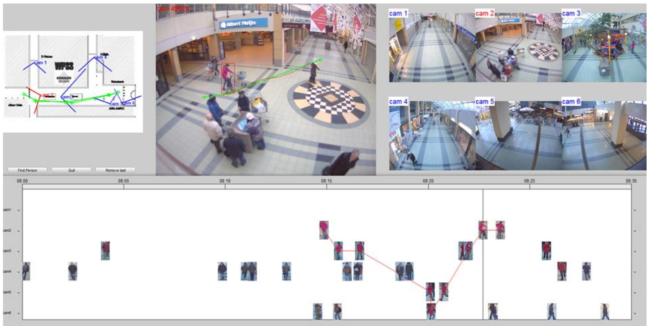
Figure 3: When searching using the re-identification engine, many candidates are suppressed and only people with similar appearance are shown. The line in the candidate panel connects the tracklets of a certain person.
