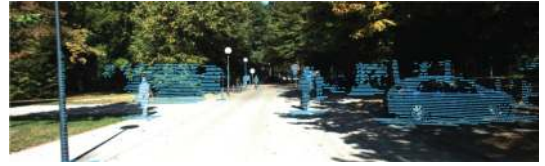
FIGURE 7: Obstacle point cloud projection image.
