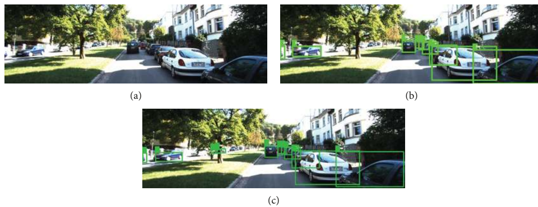
FIGURE 12: The experimental results of Scenario 1. (a) Scenario 1. (b) Results of vehicle detection using the YOLO v3 algorithm. (c) Results of vehicle detection using our algorithm.
