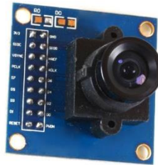
Figure 4-2 OV7670 camera module
