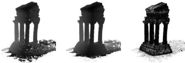
Figure 3. A stereo depth map for a dataset from [17], the fused depth map using stability-based fusion and the final confidence map (black corresponds to maximum confidence).
