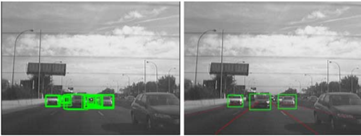
Fig. 4. Left: overlapped candidates. Right: non-maximum suppression results.
