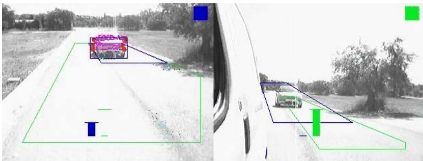
Fig. 8. Panoramic Blind Spot Detection system (Panoramic BSD)
