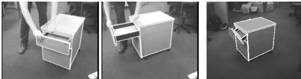
Fig. 16. Two frames from sequence tracking seven DoF filing cabinet. The third frame shows the tracker in a local minimum after relaxation of the articulation constraints.
